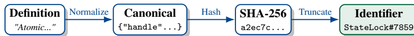
Figure 1: The content-addressing pipeline. The identifier is derived deterministically from the definition’s content.
